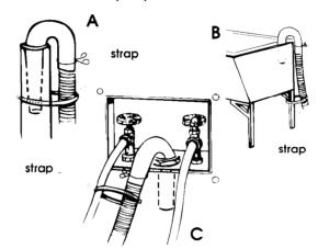
Put "hook" end of drain hose in tub or standpipe. Tightly wrap the shipping strap around the drain hose and tub or standpipe or inlet hose as shown in Figures A-C. Push plug into the nearest hole in the shipping strap.
